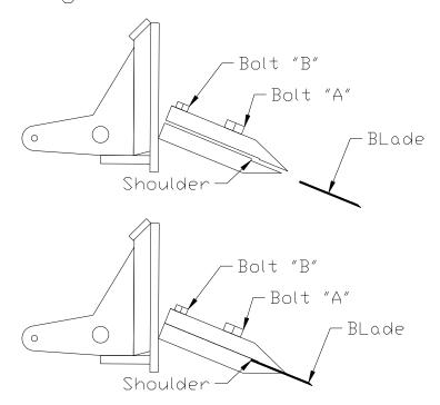
Illustration of correct scraping procedures.
